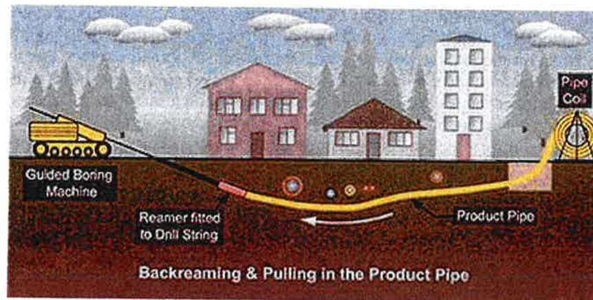
Figure 2: Backreaming and pulling the product.
